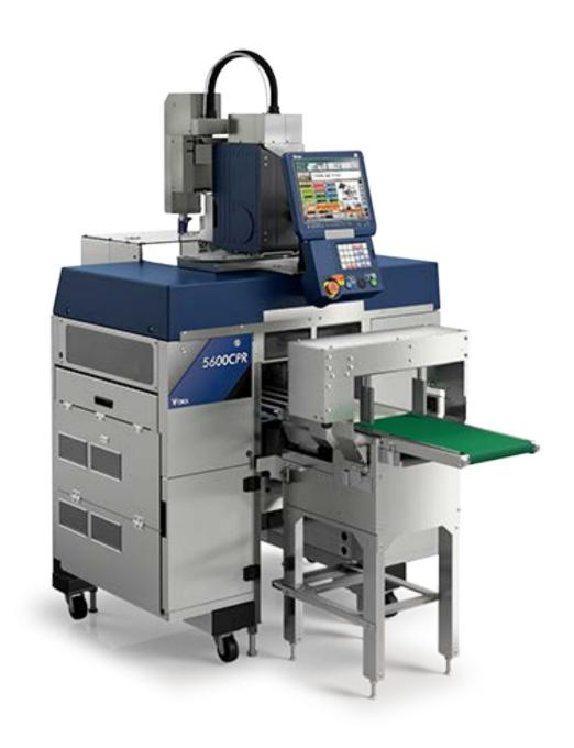
Teraoka Model AW-5600CPR-IWC Automatic Catchweighing Instrument
