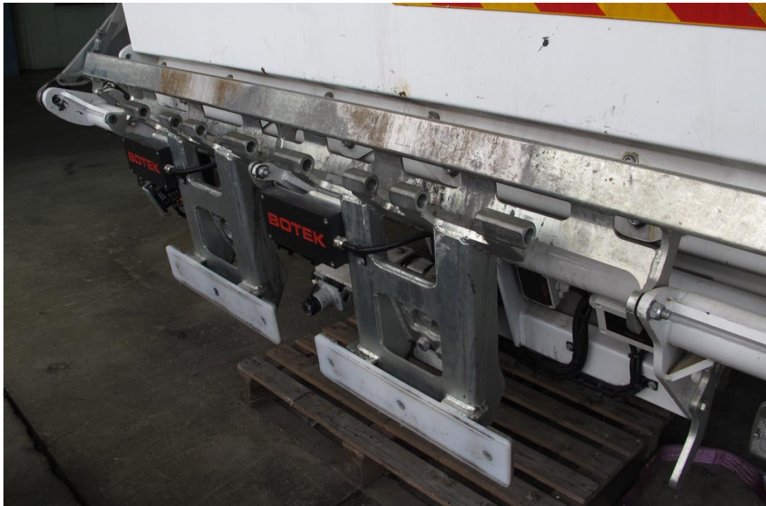
Load Cell (Installed Behind The Load Receiver Frame)
