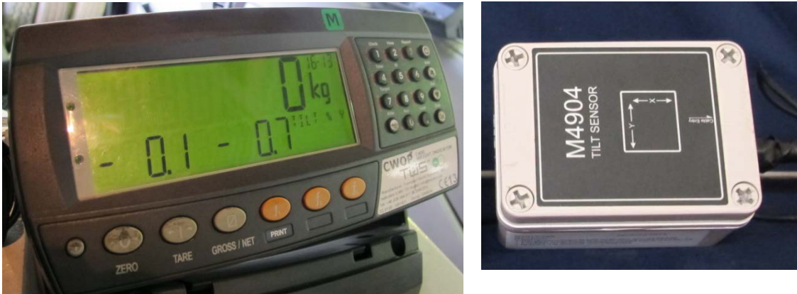
Transport World Solutions AB model CWP-C400 Digital Indicator and Rinstrum Model M4904 Tilt Sensor
