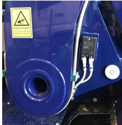
(a) Angle Sensor Located to Define Measuring Window
