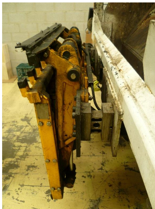
(b) Load Cell Installation
