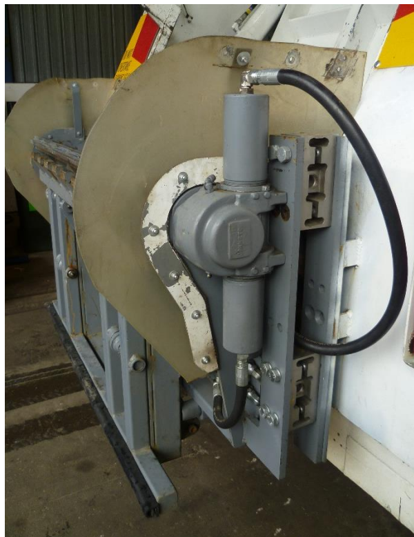
(c) Load Cell Installation
