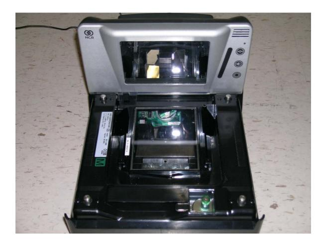
NCR Model RealScan 7874-5000 Weighing Instrument With Load Receptor Plate Removed
