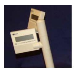
(a) Two NCR Model 7825 displays mounted on a single column
