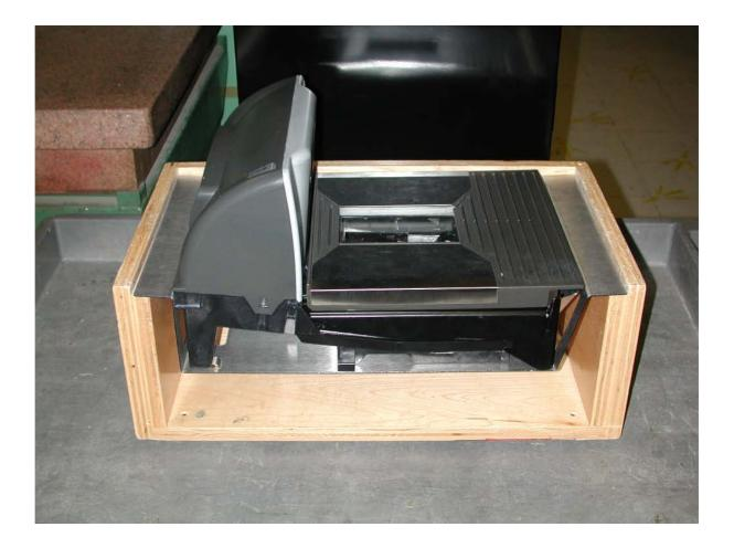
NCR Model RealScan 7874-5000 Weighing Instrument With Extended Mounting Bracket and Load Receptor
