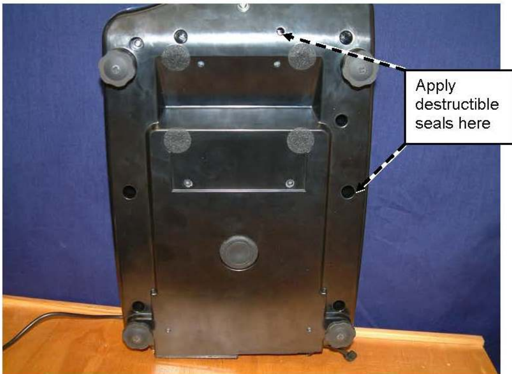
(b) Shinko Denshi (or VIBRA) CJ Series – Typical sealing arrangements
