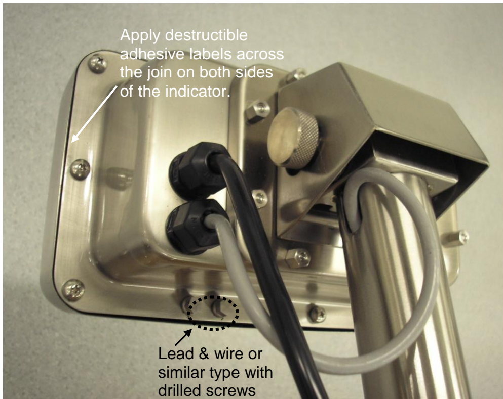
Showing Typical Sealing Methods
