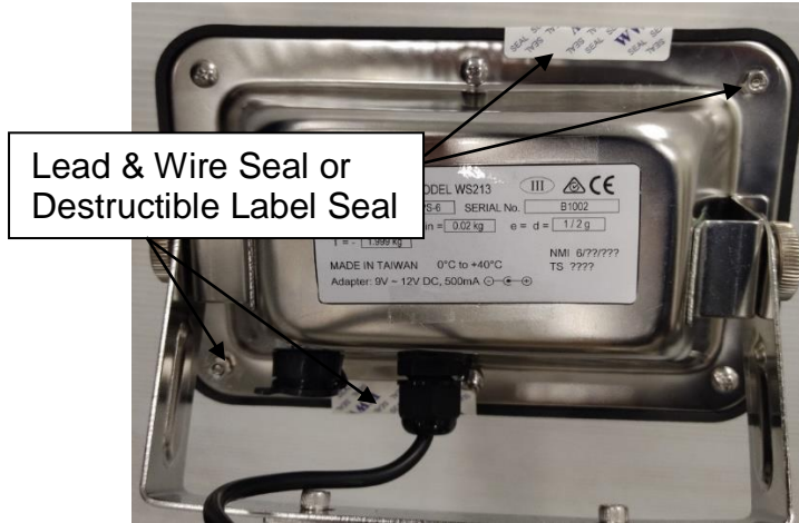
Sealing locations for Indicator
