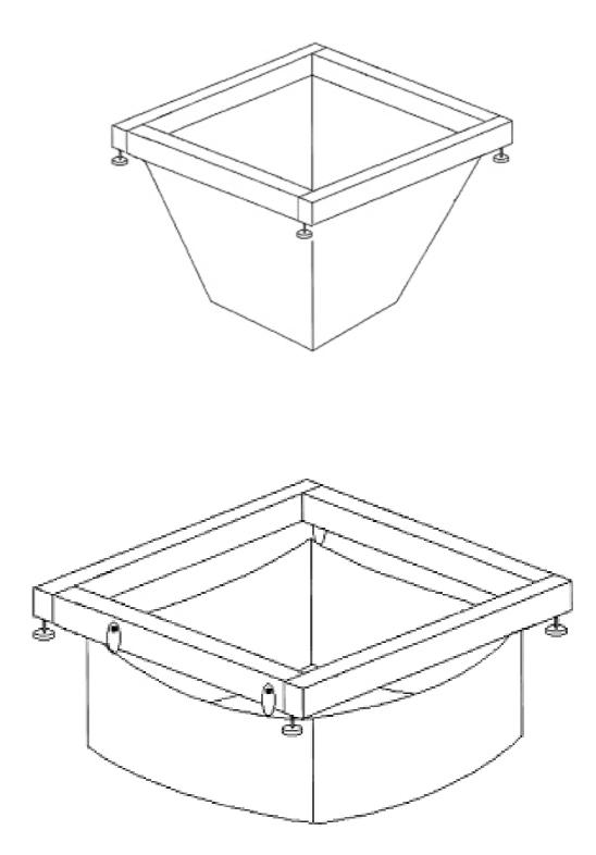
Typical HS2100 Hopper Scale Series Load Receptors
