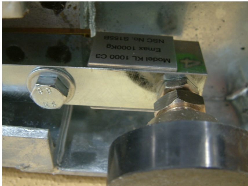
(b) Mounting for Kelba Model KL1000 C3 Load Cell
