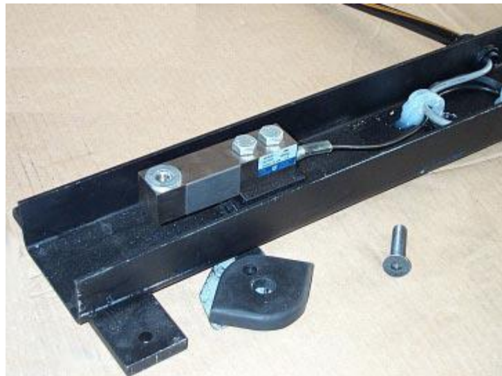
With Pairs of Load Cells Mounted in Channels (Variant 3)
