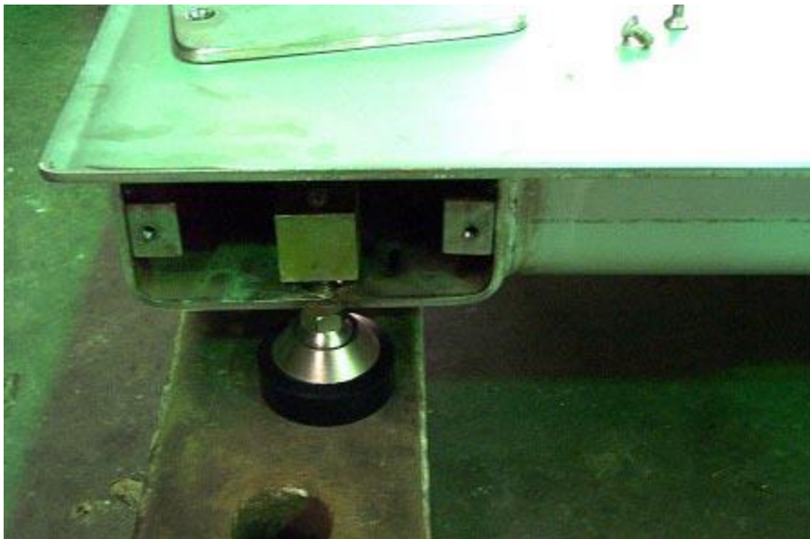
Nuweigh Model IH-1949 Weighing Instrument and Load Cell Mounting (Pattern)
