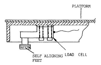
Load Cell Mountings for Variant 2 Model 7600/15 (Upper) and Model 7600 (Lower)
