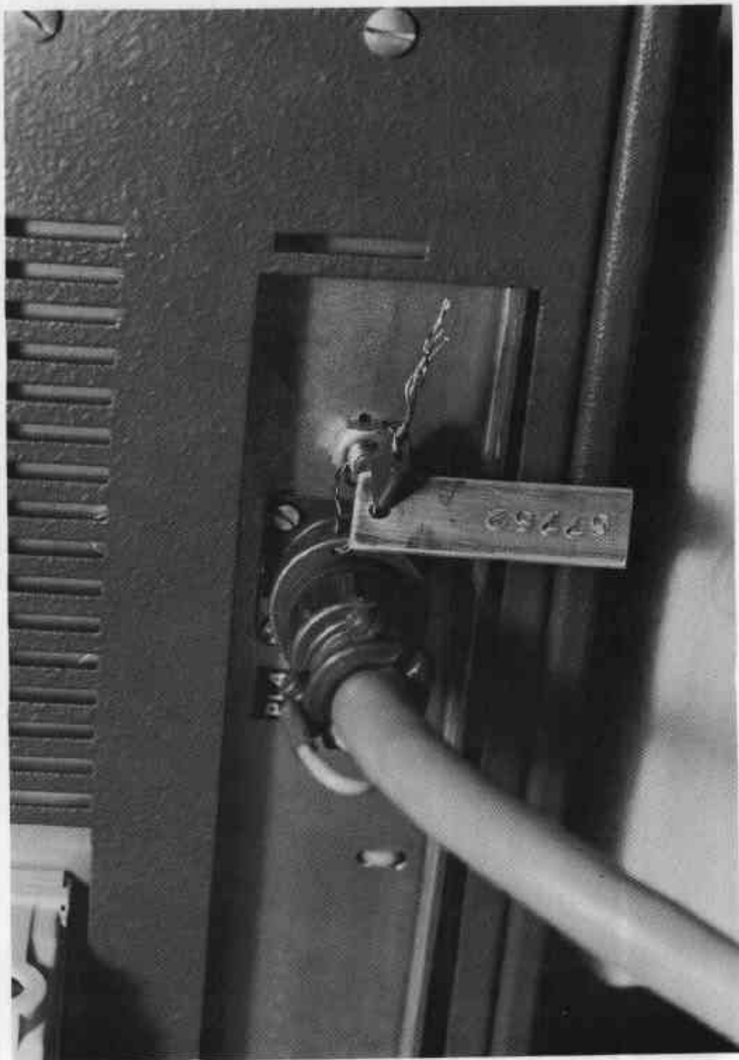
Sealing of Load-cell Cable and Load-cell Serial Number to the Weight Indicator
