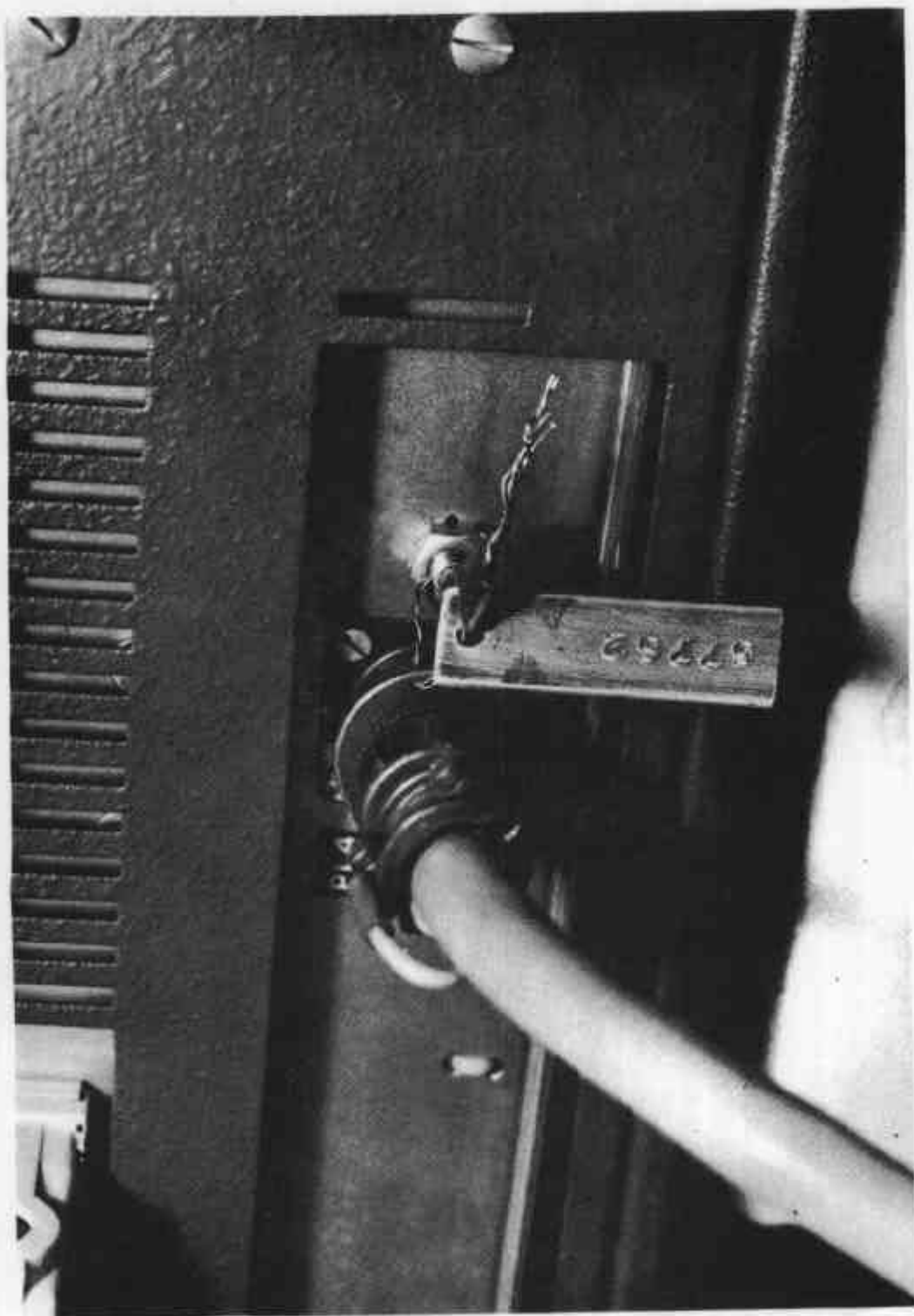
Sealing of Load-cell Cable and Load-cell Serial Number to the SB 350 Mass Indicator
