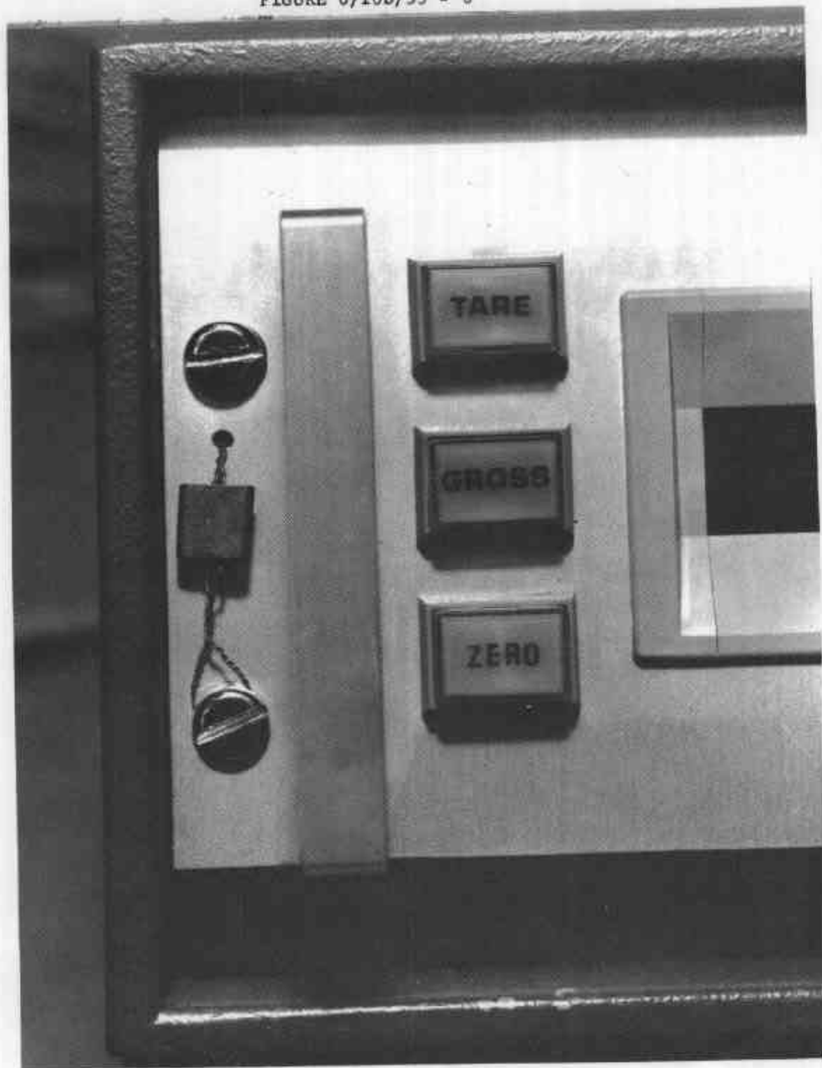
Sealing of SB 350 Mass Indicator
