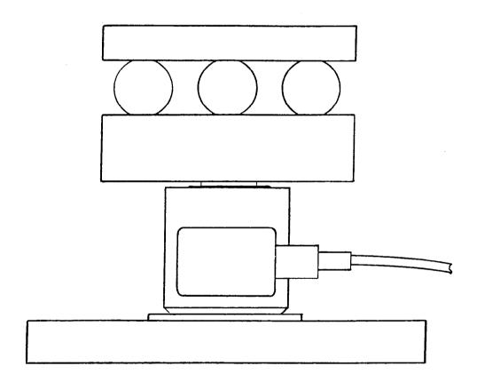
Load Cell Mounting For MW 4000 E Basework
