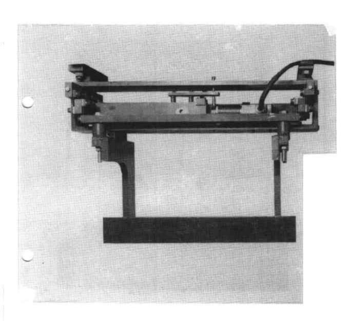
Toledo Model 2254 Overhead-track Weighing Instrument
