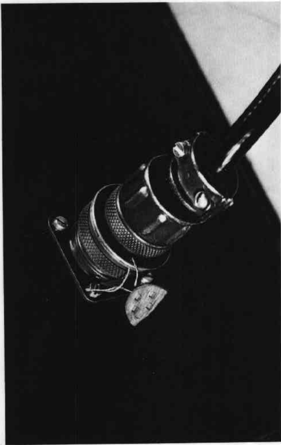
Load Cell Output Cable Showing Sealing
