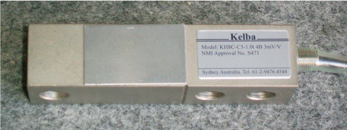
(a) Kelba Model KH8C-C3-1.0t-4B Load Cell
