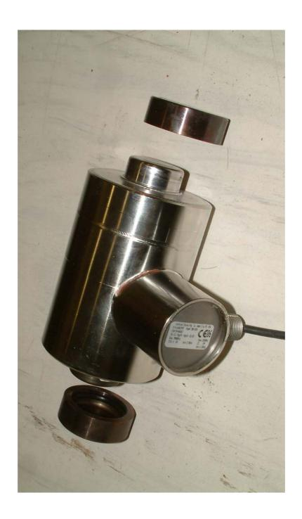
Australian Weighing Equipment Model 50K-ASCA Load Cell
