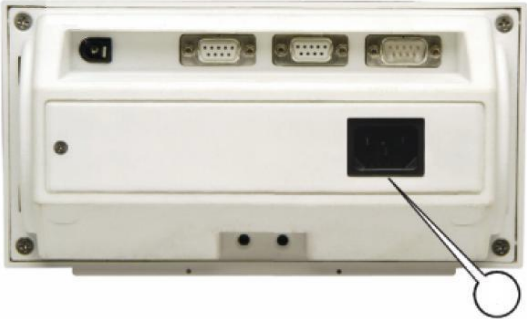
(b) Rear View – note IEC socket which distinguishes from model 70A
