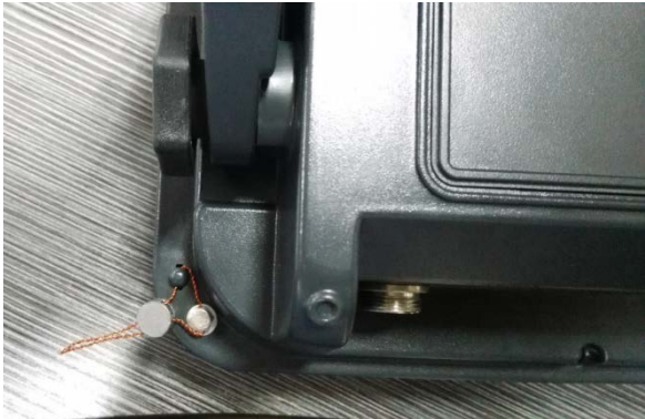
@Weigh Model NTW Digital Indicator Including Typical Sealing (Variant 4)
