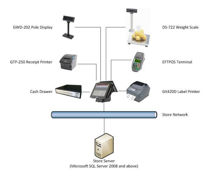
Existco Model Plant Control System V2 Point of Sale (POS) System
