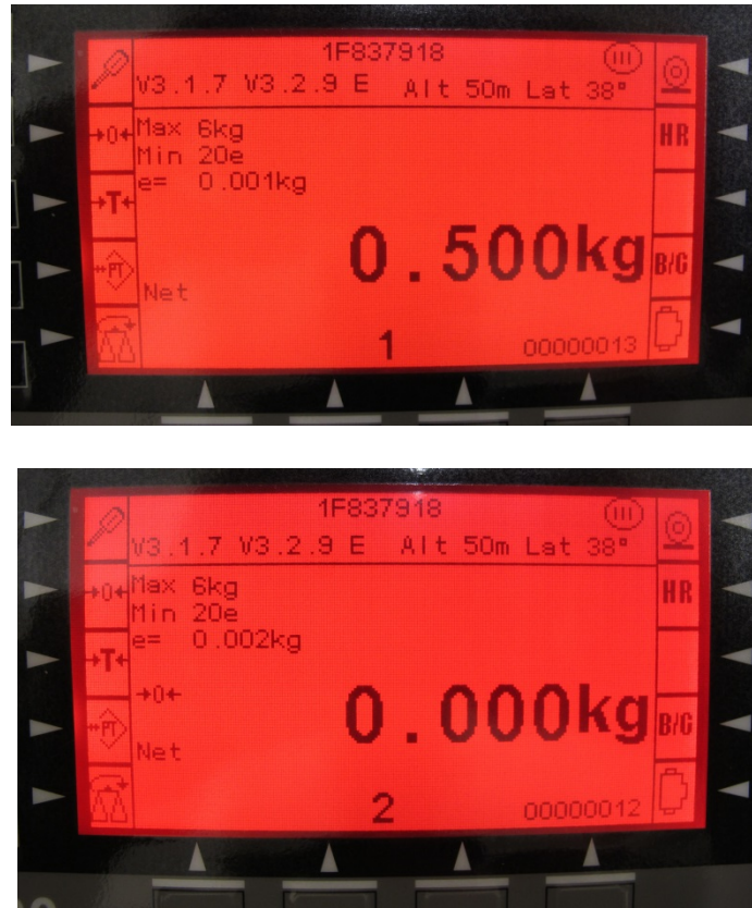
Displays From Two Platforms Connected to the Same Indicator (Variant 3)
