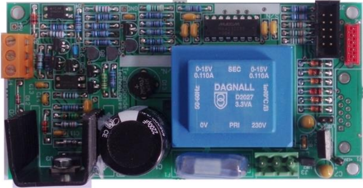
(b) Transponder Technologies Gilbarco Protocol Communication Converter
