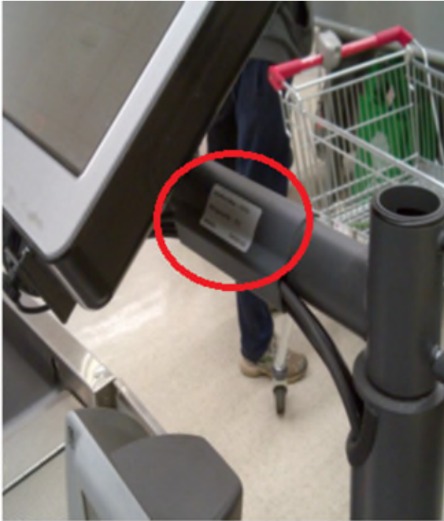
Typical Locations of Descriptive Markings
