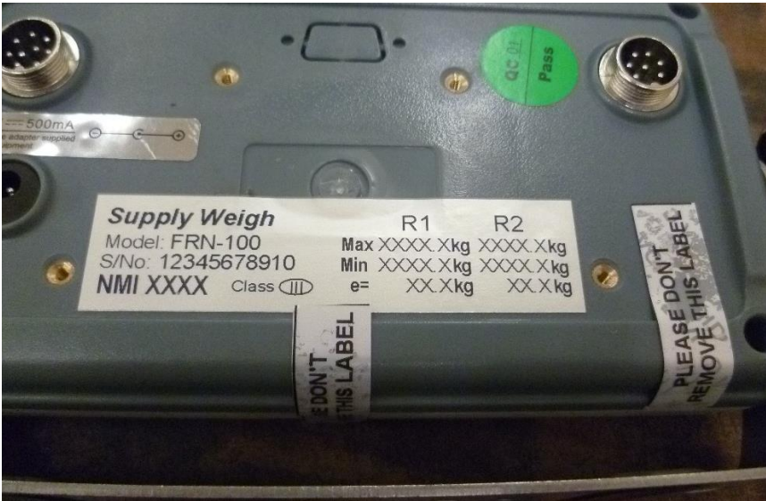
(b) Sealing with Destructible Adhesive Stickers (Variant 1)
