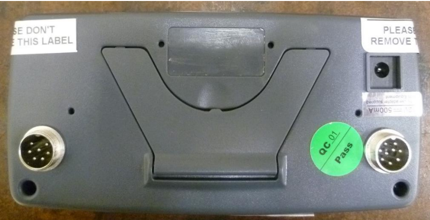
(b) Sealing with Destructible Adhesive Stickers (Variant 2)
