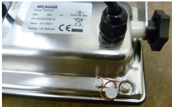
(a) Sealing of Lead and Wire Type with Drilled Screws (Pattern)
