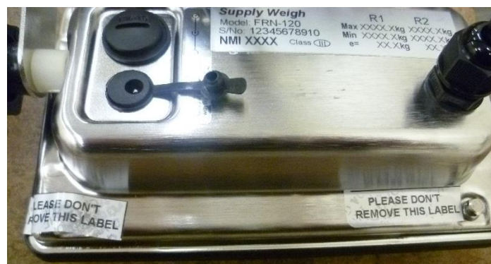
(b) Sealing with Destructible Adhesive Stickers (Pattern)
